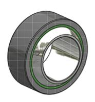
= - Dynamic load C (kN) = 1380 = - M = 50 = - O = 87.1 A = 130 Static load C0 (kN) = 2300 a (degrees) = 14 Weight (g) = 3600 B = 75
